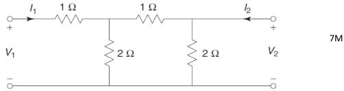
B) Find Admittance (Y) parameters for the network shown in fig.
