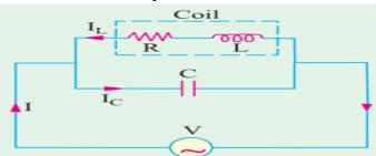
B) A coil of resistance  $20~\Omega$  and inductance  $200~\mu H$  is in parallel with a variable capacitor. This combination is in series with a resistor of  $8000~\Omega$ . The voltage of the supply is 200~V at a frequency of 106~Hz. Determine (i) the value of C to give resonance (ii) the Q of the coil (iii) the current in each branch of the circuit at resonance.
